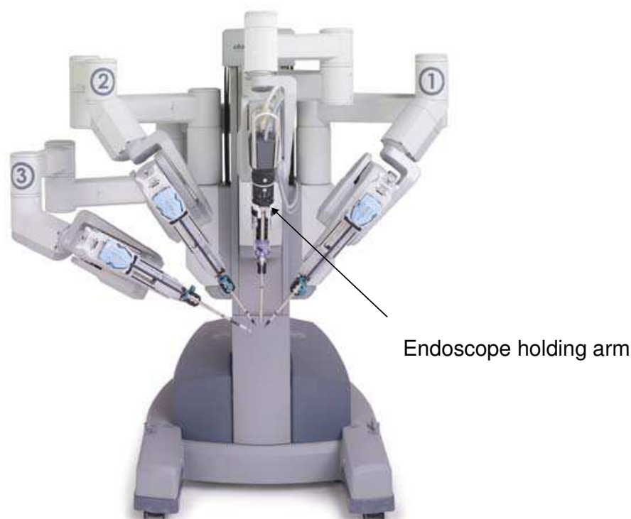
Fig. 7. Robotic cart has one endoscope holding arm and three surgical arms.
