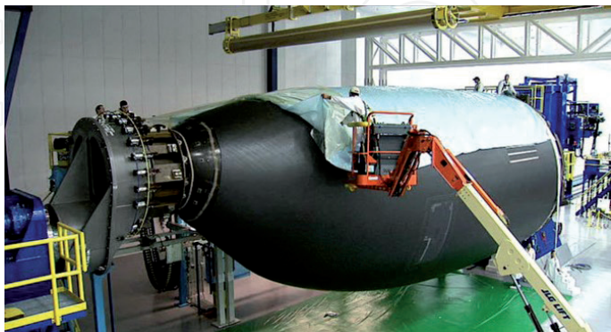
Figure 17. OML sector panel tool. Source: Premium Aerotec.
