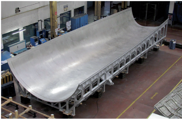
Figure 17. OML sector panel tool. Source: Premium Aerotec.
