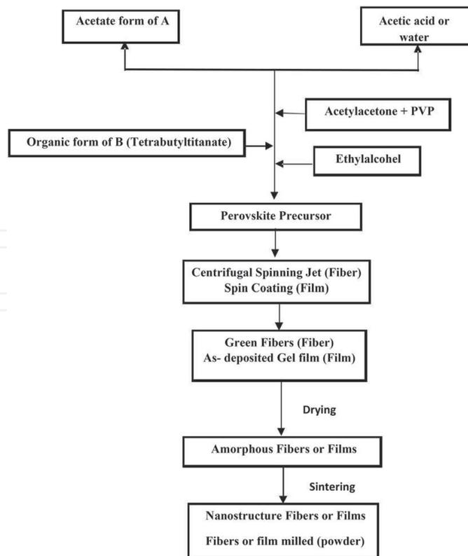
**Figure 4.** The preparation process of nanostructured  $ABO_3$  fibers, film, and powder by the sol-gel route (Habibollah Aminrastabi Method).
