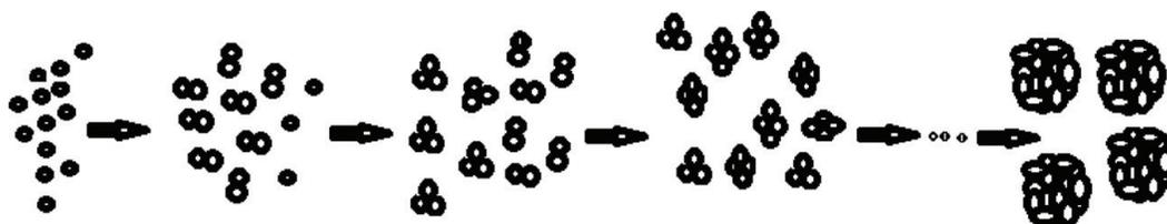
Figure 3. Schematic bottom-up and dynamic assembly of grain during the synthesis process.
