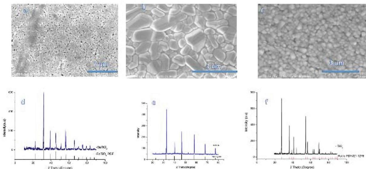
**Figure 7.** SEM images and XRD patterns of different layers sintered at different temperatures and soaking times: (a and d)  $BaTiO_3$   $900^\circ C$  for 120 min, (b and e)  $SrTiO_3$   $1100^\circ C$  for 120 min, and (c and f)  $TiO_2$   $900^\circ C$  for 120 min.
