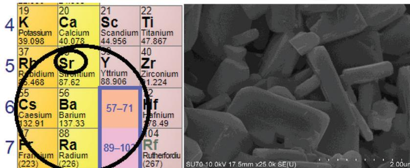
**Figure 8.** SEM micrograph of  $(Ba_{0.95}Sr_{0.05})TiO_3$  with microstructure cubic grain.
