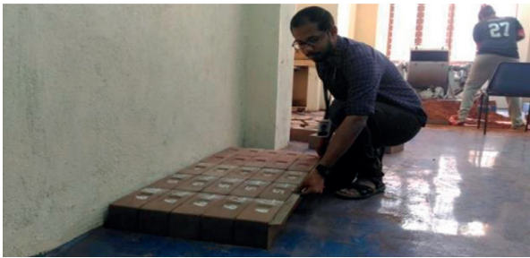
Figure 3. Dimensionality test of geopolymer bricks.
