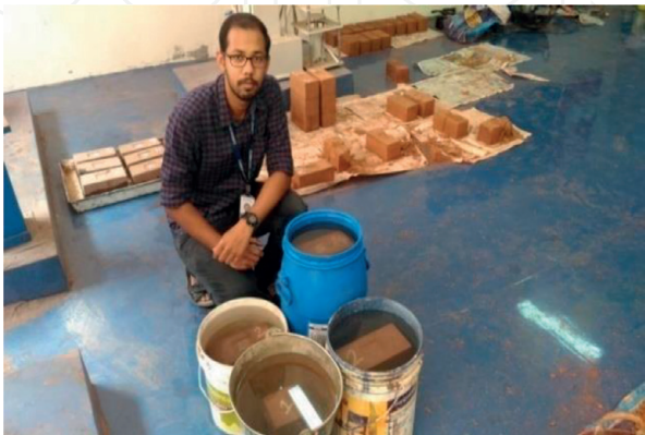
Figure 2. Water absorption test of geopolymer bricks.
