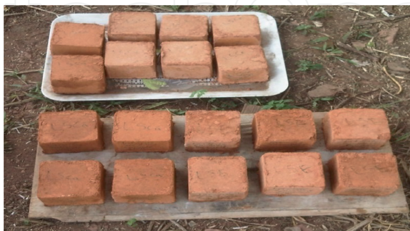
Figure 11. Samples of nonconventional clay bricks. Source: [33].
