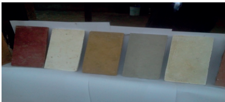
Figure 14. Samples of cement-bonded Cissus populnea fibre-reinforced floor tiles produced. Source: [41].
