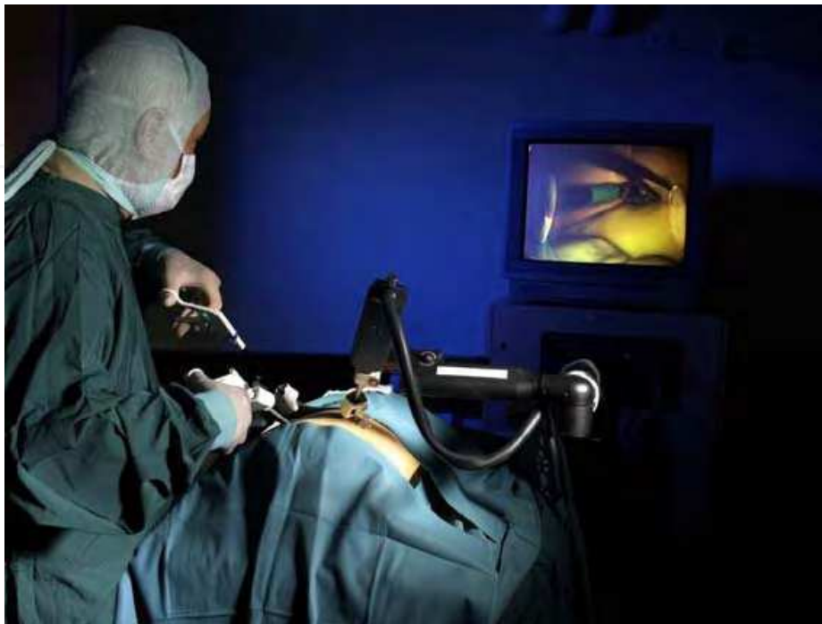
Figure 8. DLR automated camera guidance scenario with AESOP robot
