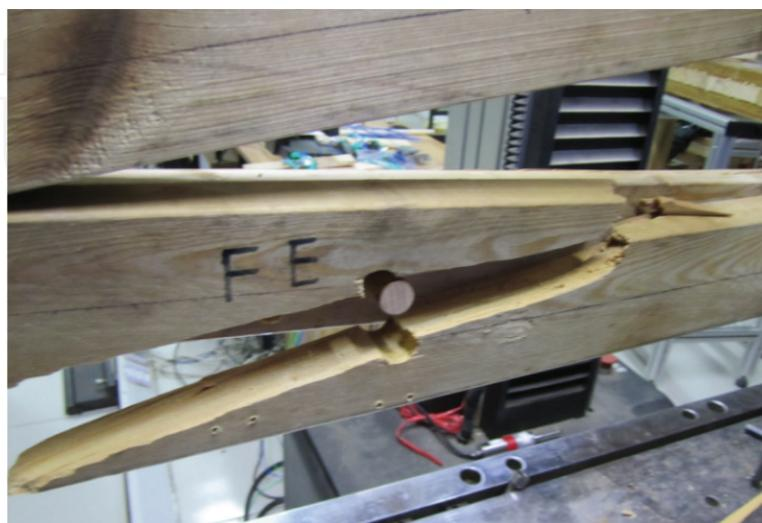
**Figure 11.** Failure phenomenon of SPT-G2-20-1.
