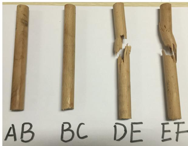
**Figure 19.** Failure of connectors in SPT-G3-16.
