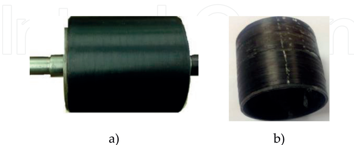
Figure 1. Rotor (a) with a rotor sleeve made of composite material (b).
