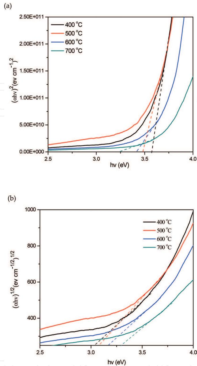
**Figure 8.** (a) Plot of  $(\alpha hv)^2$  as a function of photon energy (eV) and (b) Plot of  $(\alpha hv)^{1/2}$  as a function of photon energy ( $h\nu$ ).
