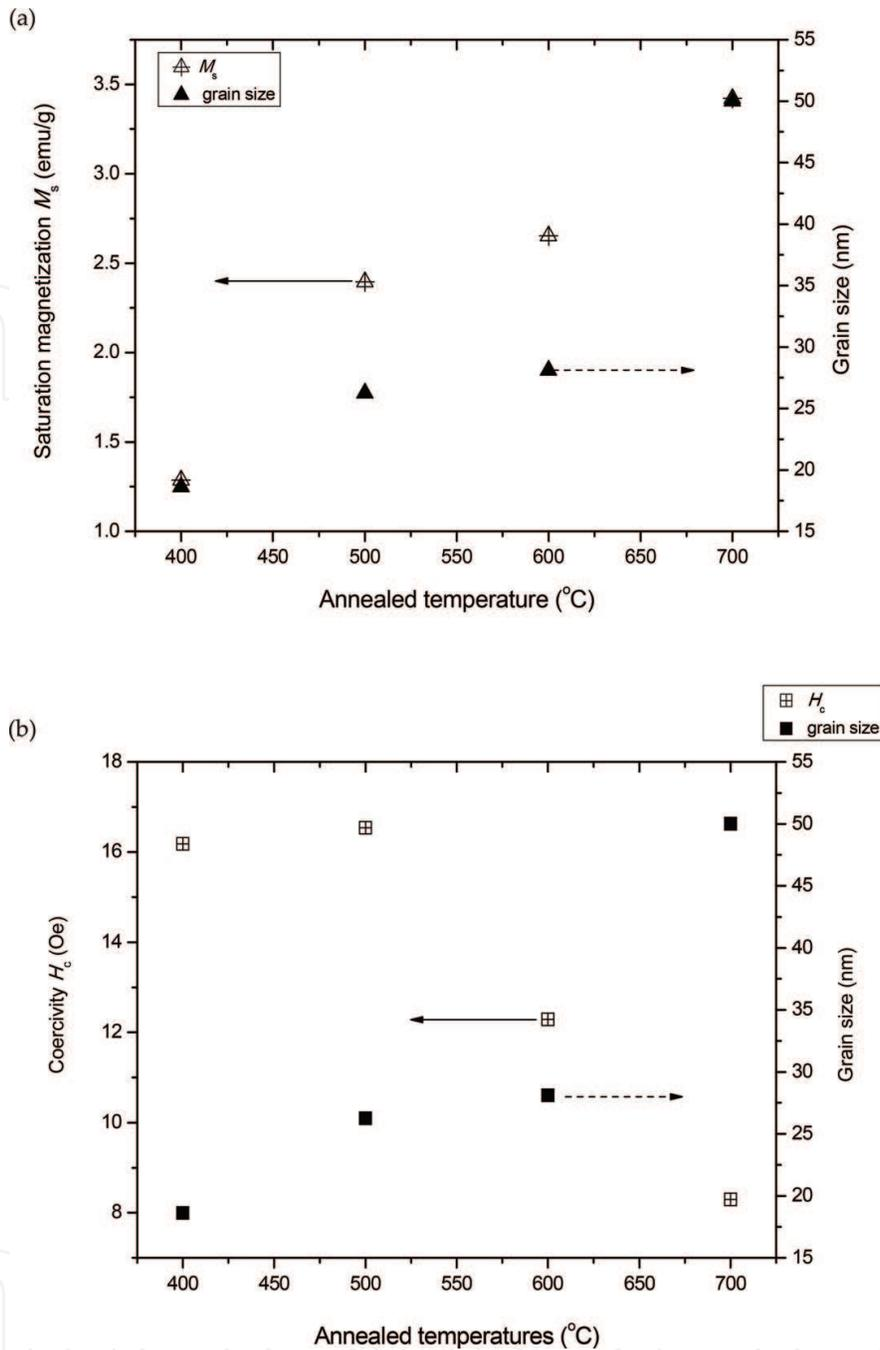
**Figure 6.** Comparison of the variation in (a)  $M_s$  and (b)  $H_c$  as a function of annealed temperatures of the  $\text{Ni}_{0.3}\text{Zn}_{0.7}\text{Fe}_2\text{O}$  nanoferrite thin films. Reproduced with permission from [21].
