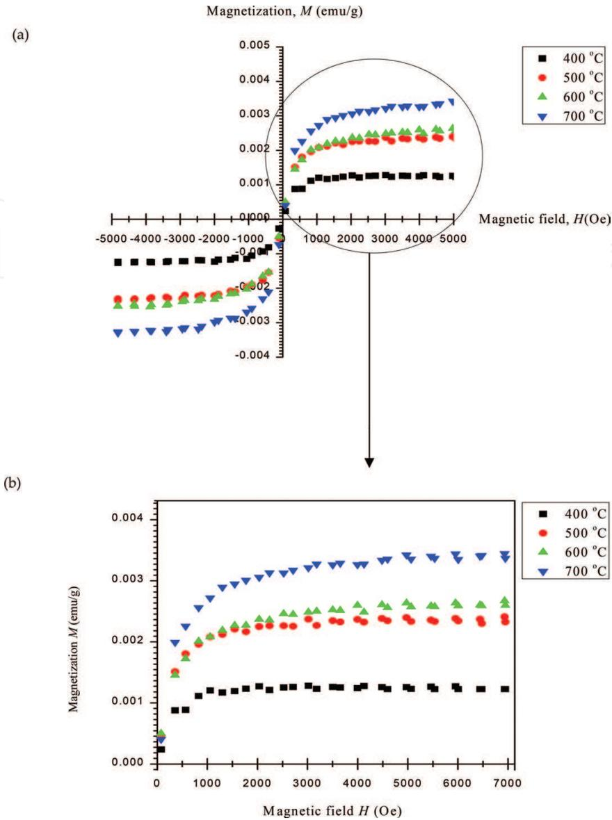
**Figure 5.** (a) Hysteresis loop of Ni<sub>0.7</sub>Zn<sub>0.3</sub>Fe<sub>2</sub>O<sub>4</sub> ferrite thin films and (b) first quadrant of the magnetic hysteresis loops of the samples. Magnetization at any given field increased with heat treatment temperature. Reproduced with permission from [21].
