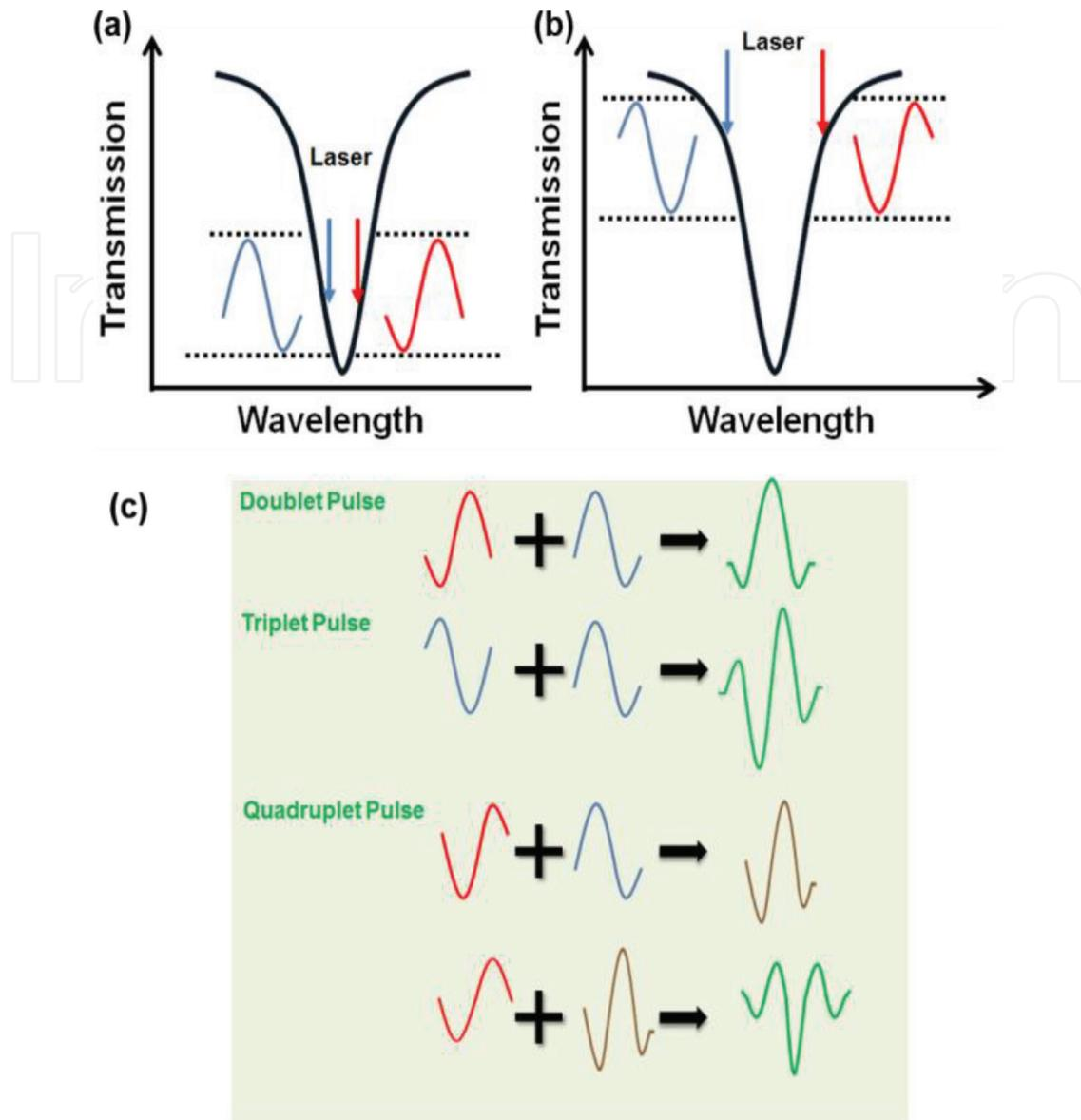
**Figure 2.** The schematic diagram of the (a and b) generation of asymmetric monocycle pulses; (c) generation of higher-order Gaussian pulses using combination of different asymmetric monocycle pulses.
