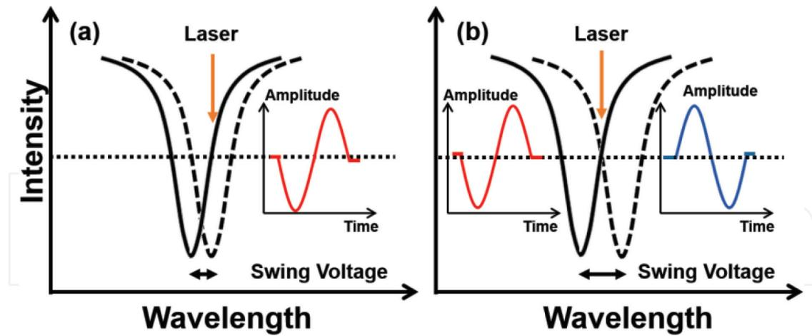
**Figure 12.** The schematic principle of the tunable-filter-based (a) UWB OOK modulation and (b) UWB biphase modulation.
