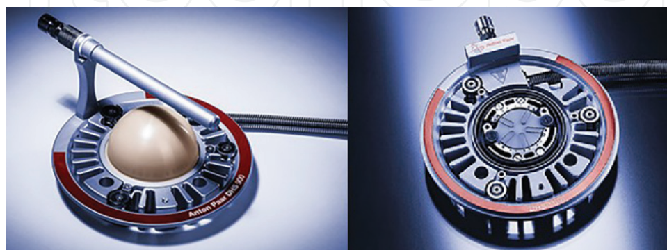
Figure 4. Oven coupled to the X-ray diffractometer.
