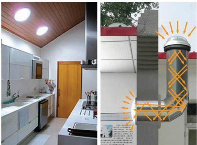
Figure 9. Solar light pipes system. Source: Google Search—Images.
