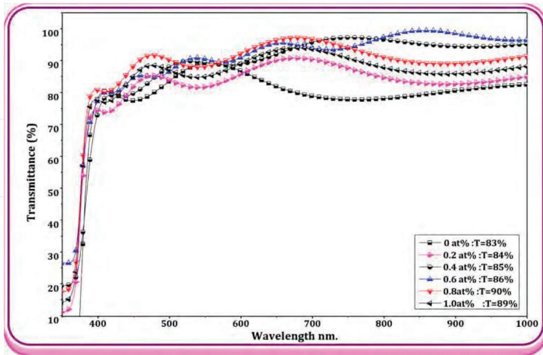
Figure 13. Percentage transmittance of ZnO doped with different % of boron.
