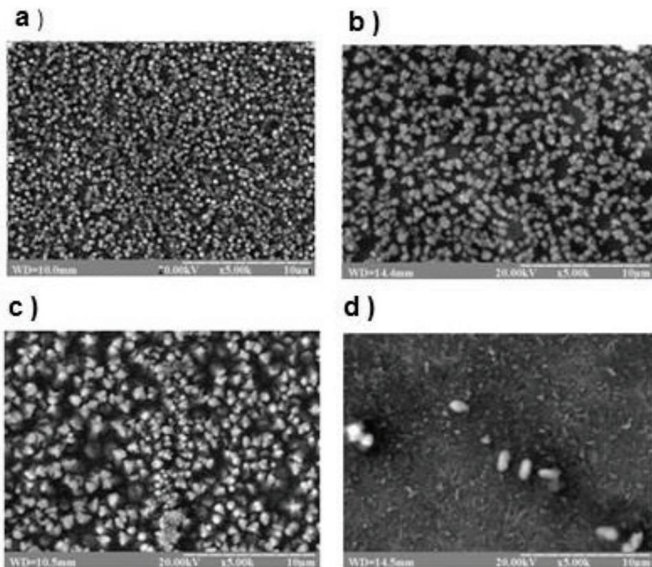
**Figure 4.** SEM morphological structure of Cu-doped ZnO thin film [a–d] as deposited and annealed at temperature; 500, 700 and 850°C.
