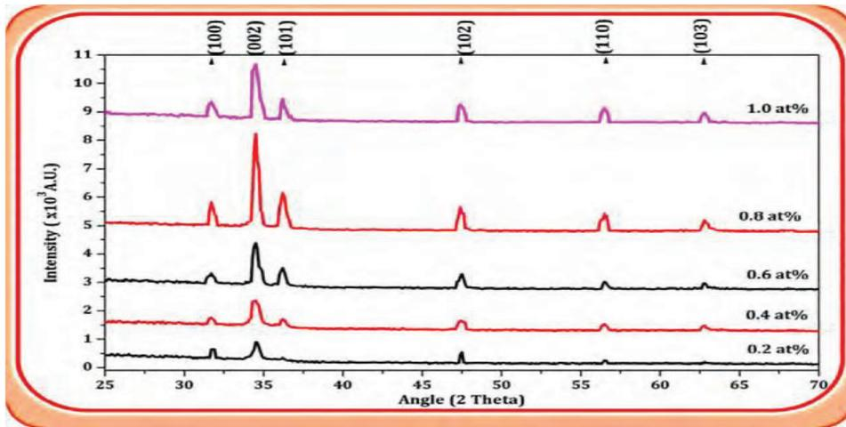
Figure 8. XRD spectra for various percentage boron doped ZnO thin film.
