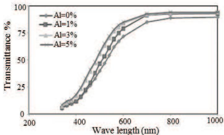
Figure 12. Percentage transmittance of ZnO doped with % aluminum.
