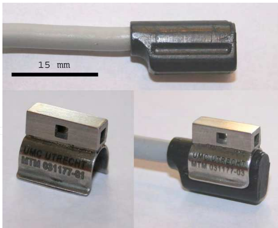
Figure 1. Thirteen MHz epicardial ultrasound mini-transducer (upper panel), custom made snap-on metal clip (left lower panel) and clip attached to mini-transducer (right lower panel). The clip is designed specifically for easy handling of the mini-transducer by the end-effectors of the robot instruments
