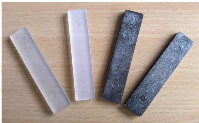
Figure 1. Injected specimens of PP and a PP-bagasse biocomposite.
