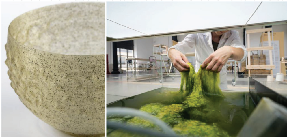
Figure 2. 3D printed cup with algae-based filaments (right), realized by Luma Foundation in collaboration with Musée Départemental Arles antique; (left) sample of Cladophora macroalgae [21].
