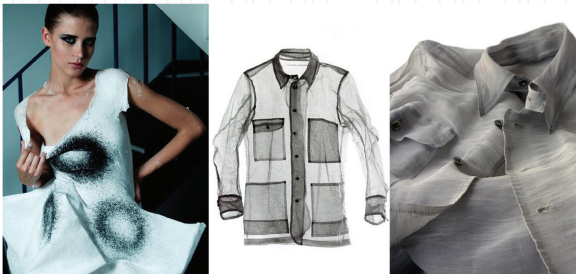
Figure 1. Dress realized with the sprayable textile technology [14], and the “Oricalco” shape-memory shirt [15].
