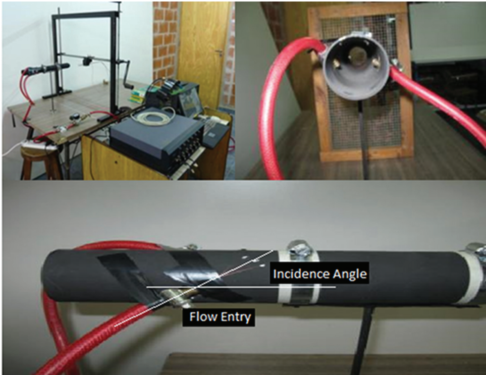
Figure 13. Experimental set-up for longitudinal vortex generation.
