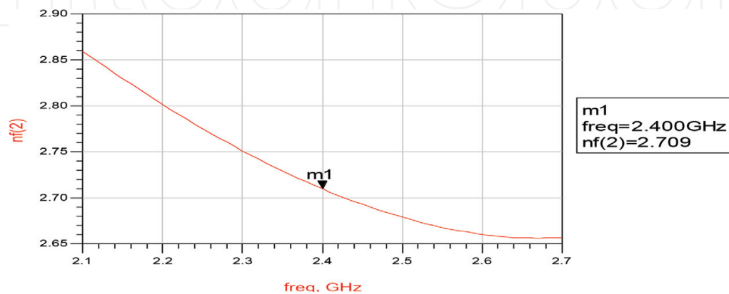
Figure 17. NF of DDC LNA.
