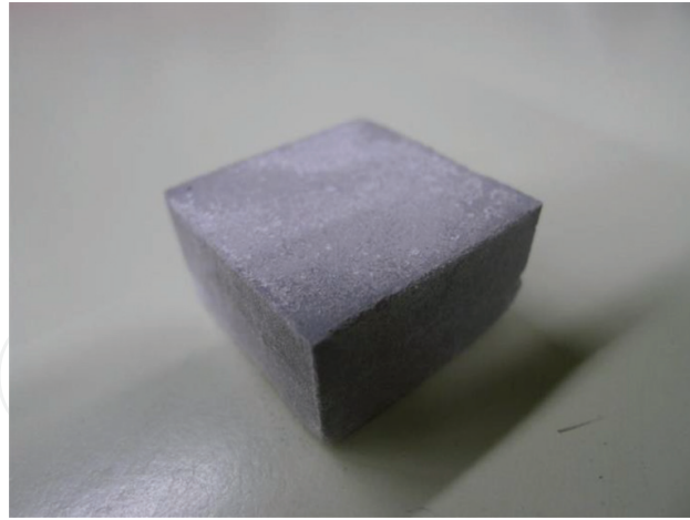
Figure 4. Magnesium hydride (the external size of 35 × 35 × 17 millimeter, Bio-Coke Ltd. Japan).
