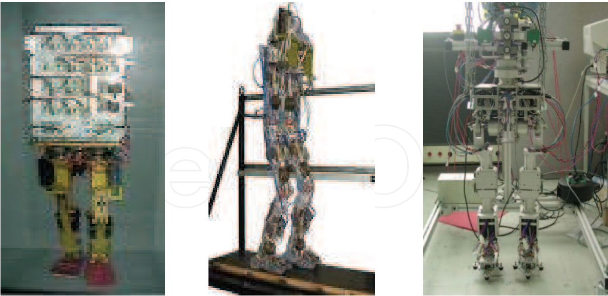
Fig. 2. Humanoid locomotion systems or biped robots, (a) BIP robot, (b) Lucy robot, (C) Robian robot.
