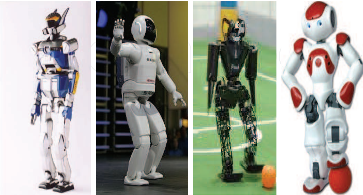
(a) 2 (b) 3 (c) 4 (d) 5 Fig. 1. Humanoid robots: (a) and (b) are human size robots, (c) and (d) are middle size robots. (a) HRP2, (b) ASSIMO, (c) Nimbro soccer robot, (d) NAO robot.
