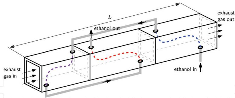
Figure 5. Exhaust gas recirculation heat exchanger modular design.
