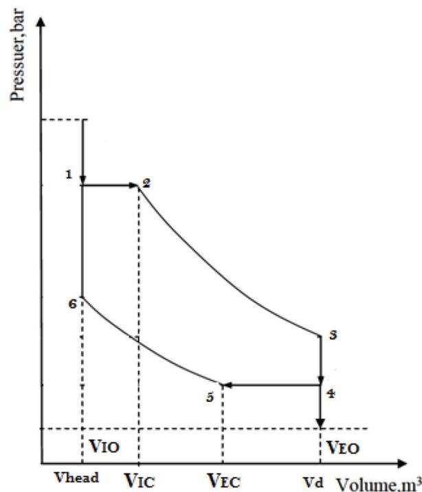
**Figure 3.** p-V diagram of the expansion process ( $V_2 = V_{IC}$ : intake valve closing volume;  $V_5 = V_{EC}$ : exhaust valve closing volume;  $V_{head}$ : clearance volume;  $V_d$ : displacement volume).
