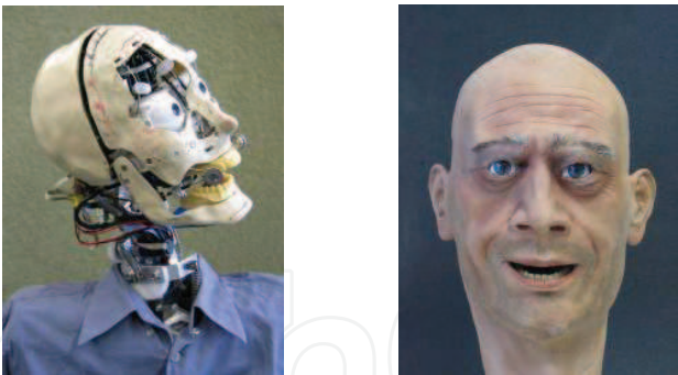
Fig. 1. The social interactive humanoid robot ROMAN, left: bare head, right: silicon skin clued on the head
