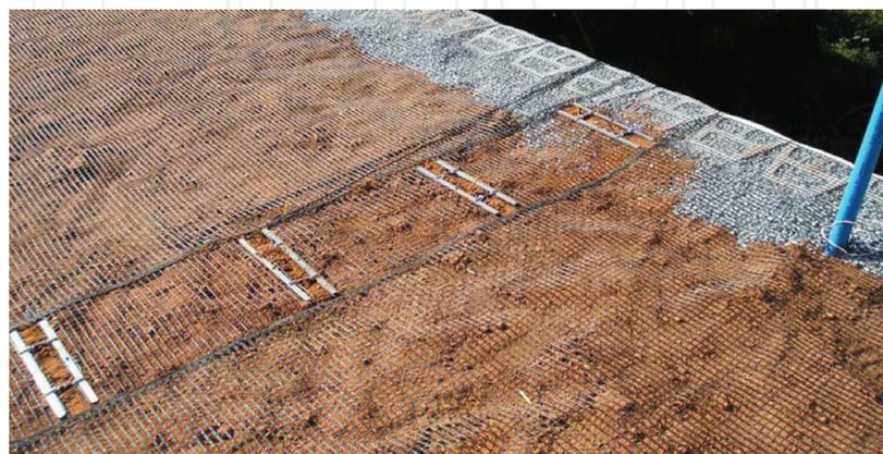
Figure 7. Load cells positioned along the reinforcement [21].
