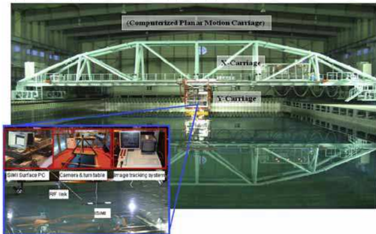
Fig. 8. CPMC and image tracking system of the OEB.
