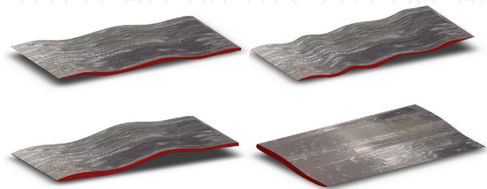
Figure 10. Extracted shape of deformed strands in COSB.
