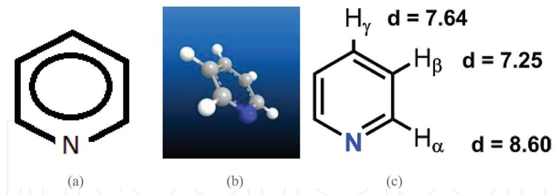
**Figure 1.** (a) The double bonds in pyridine are shared between all of the atoms in the circle so that they can be drawn as a circle instead of individual bonds. (b) Pyridine. (c) The hydrogen atoms on pyridine have three distinct chemical shifts. Pyridine shares the electrons in the entire circle, but the nitrogen draws more electrons to it, causing a slight dipole to form.
