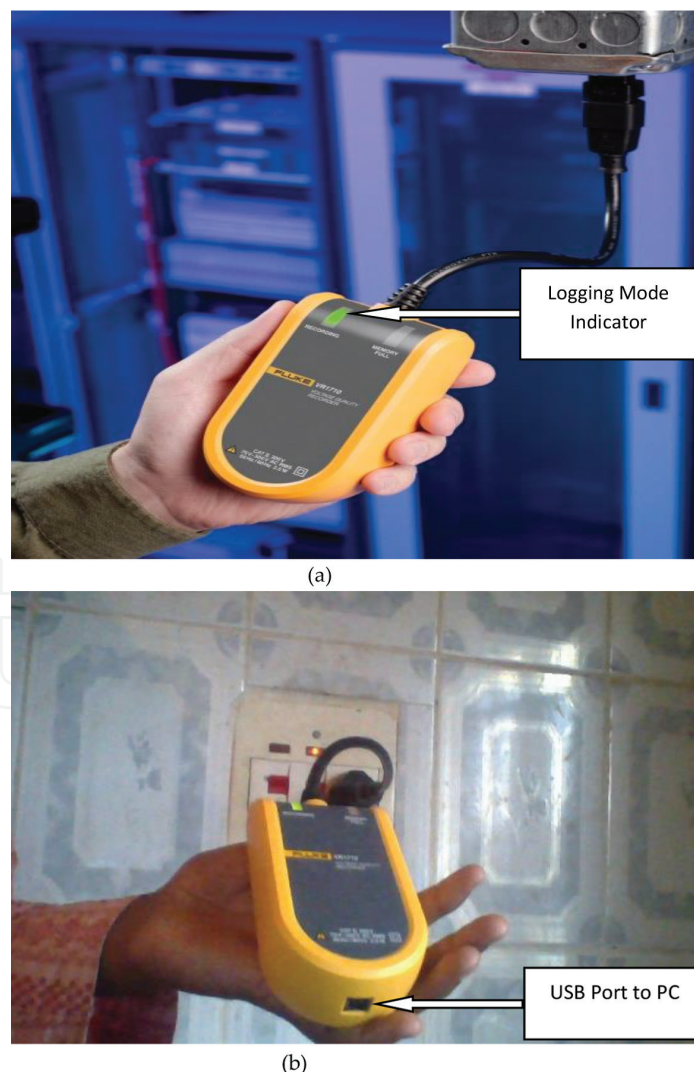
Plate 1. Voltage quality recorder (VR1710) logging data. (sources: (a) installation manual of fluke VR1710 (b) at a residential power outlet in Bauchi).
