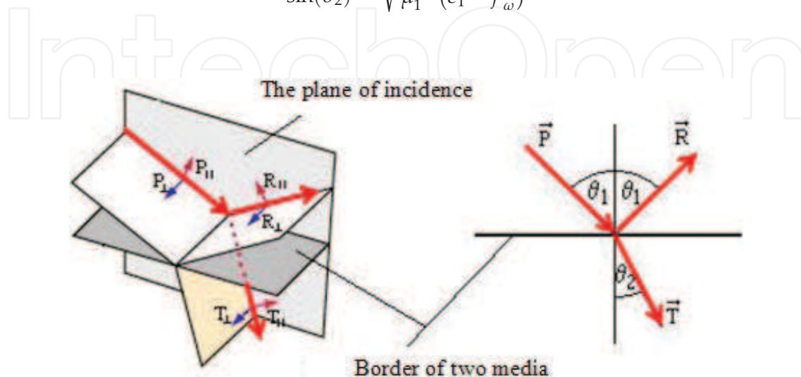
**Figure 8.** The EM wave reflection and transmission phenomenon.
