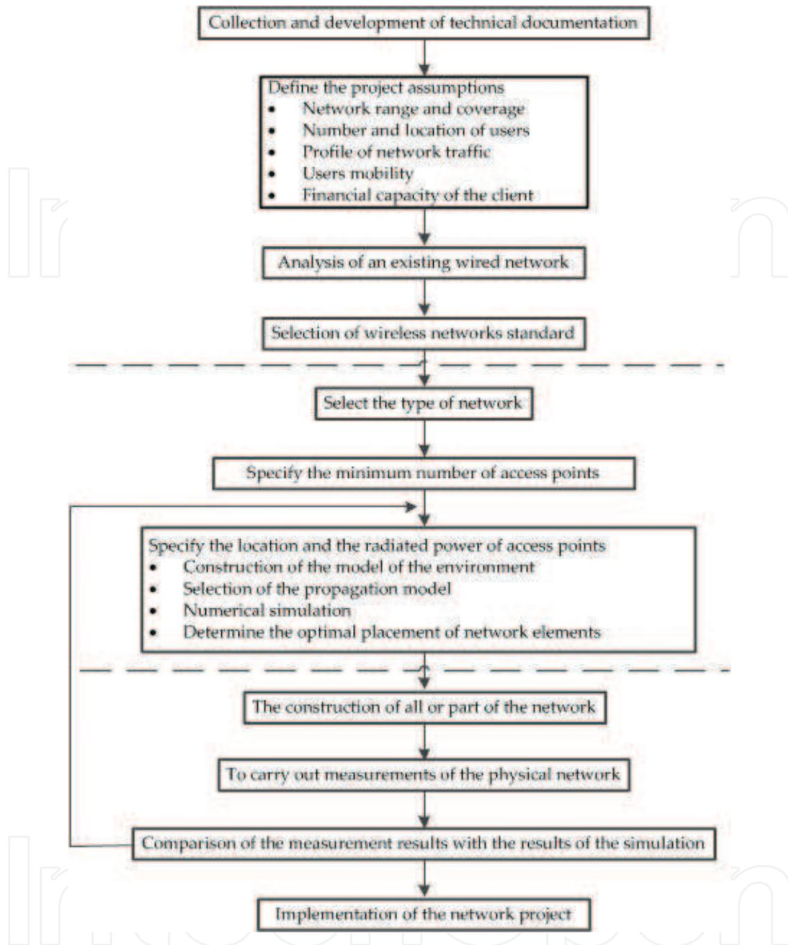
Figure 11. Design algorithm of wireless communication networks.
