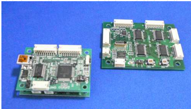
Fig. 5. Sensor controller and driver consisting of dsPIC board and extension board
