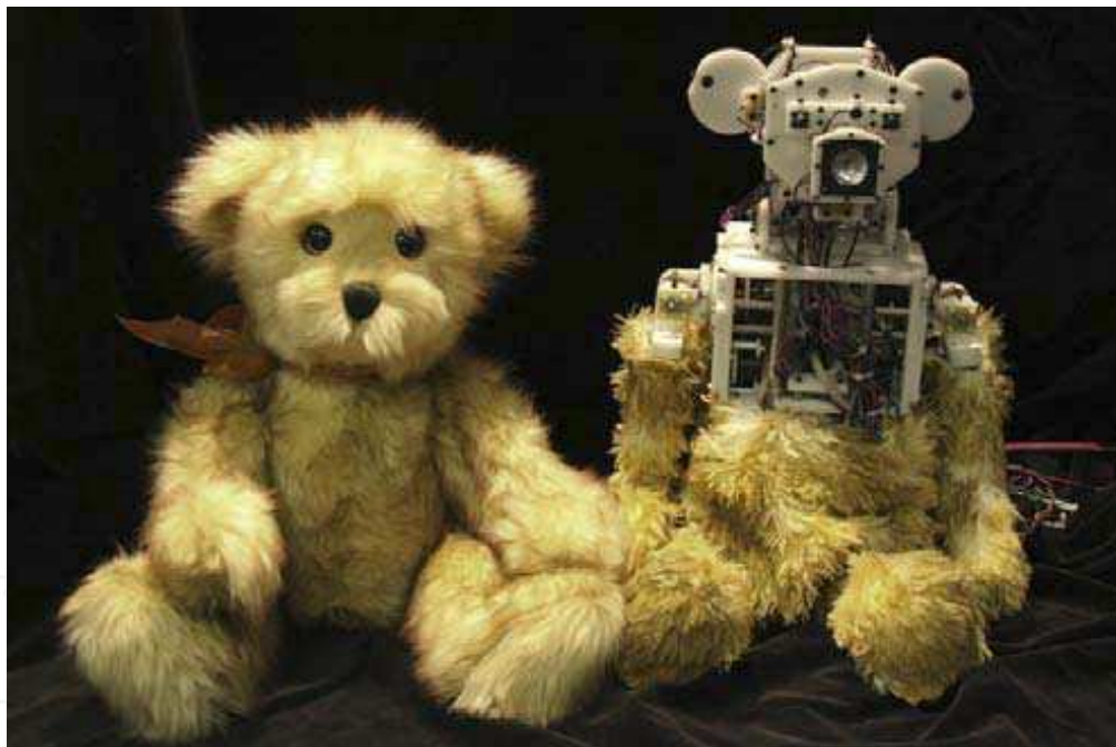
Fig. 2. The Current Huggable V3.0 Prototype (in development) (right) and the Concept Plush by Tammy Hendricks (left). In the current prototype only the underlying mechanics of the robot are shown. The sensitive skin system, soft silicone rubber synthetic skin, and final cosmetic fur exterior are not shown in this photo. When fully finished the Huggable robot will look like the concept plush at left.
