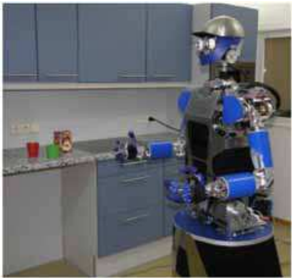
Fig. 11. The Humanoid robot ARMAR-III (Asfour et al., 2006).
