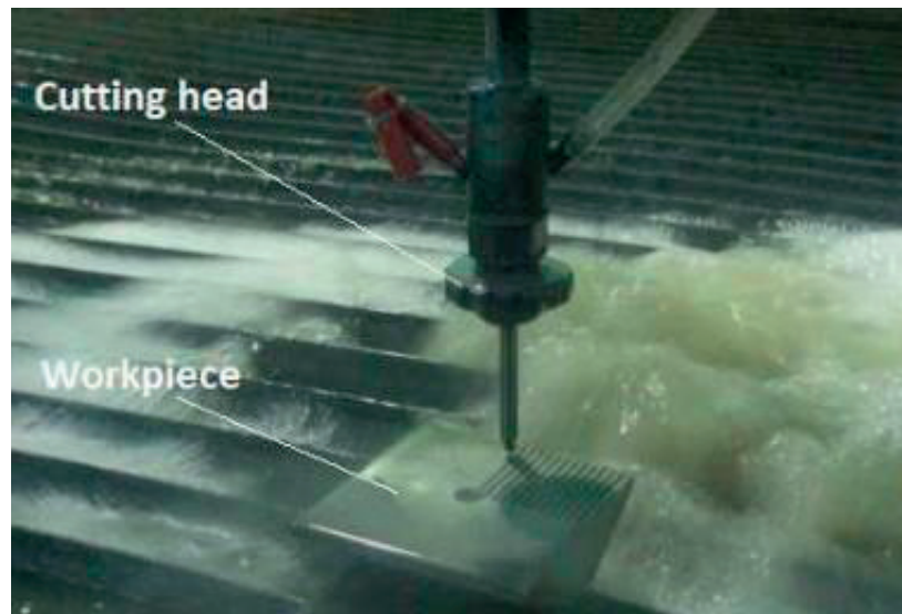
Figure 4. Experimental setup for determination of maximum depth of cut.
