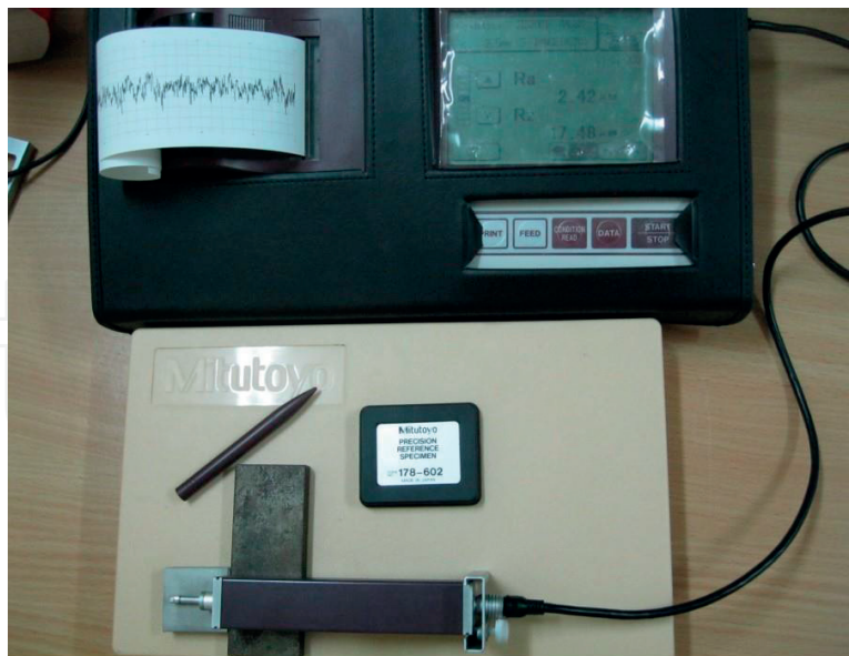
Figure 7. Measurement of surface roughness.
