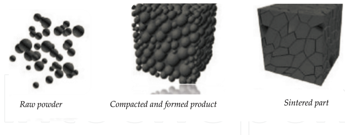
Figure 3. Powder to bonded structure during sintering.
