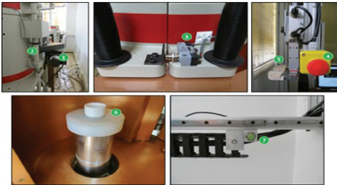
Figure 23. Positioning system: 1. Electric motor to open/close shielding; 2. Shield sensor for opening; 3. Shield sensor for closing; 4. Emergency stop; 5. Sample gripper; 6. Detector sample support; 7. Actuator motion limit sensor.
