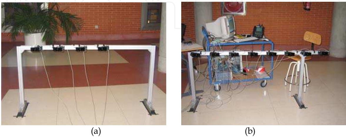
Fig. 12. IR barrier prototype: (a) Emitter barrier; (b) Receiver barrier.
