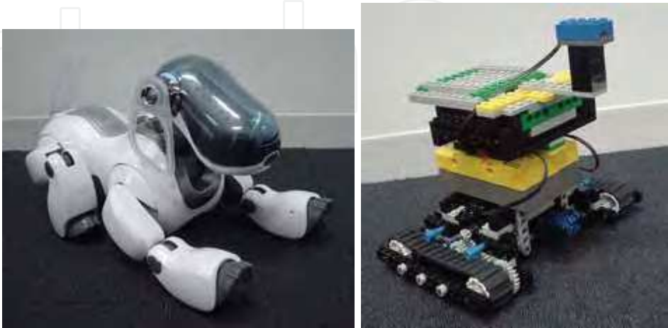
Figure 2. The appearances of AIBO (left) and MindStorms (right)
