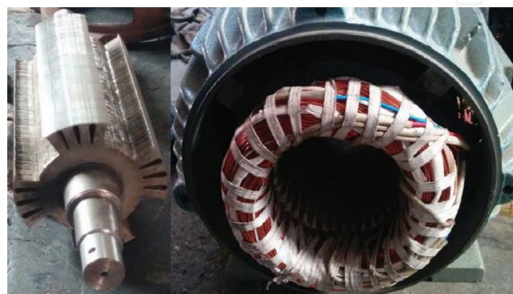
Figure 11. Fabrication details of 6-4-2 BDFRM.
