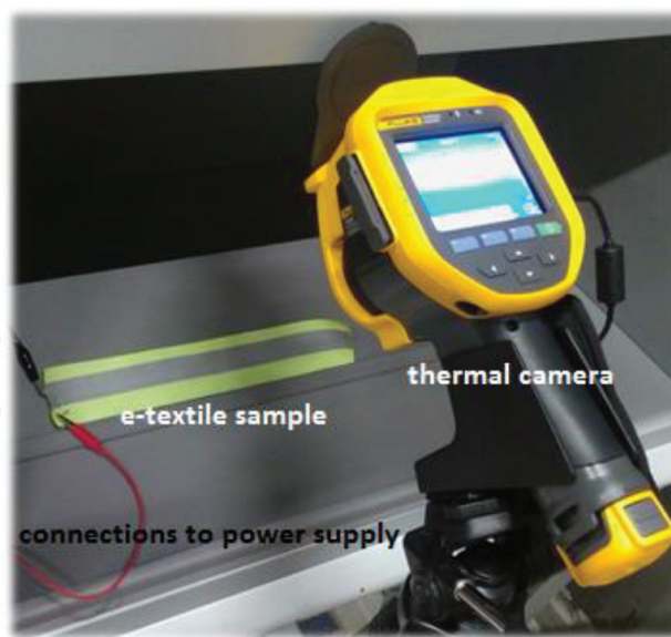
Figure 10. Testing set up to measure surface temperature.
