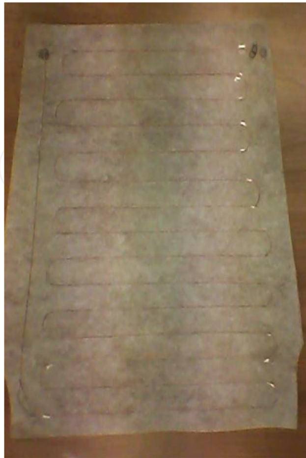
Figure 12. Placement of conductive yarn over interlining.
