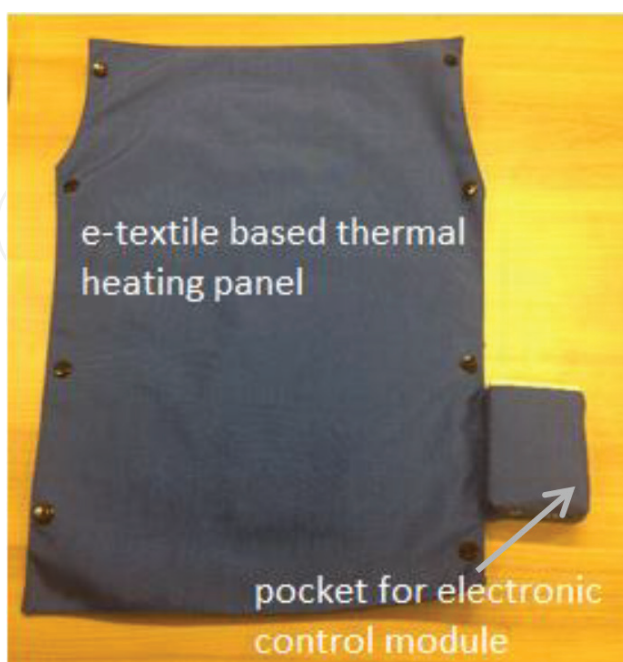
Figure 16. Insertion of electronic control module inside the pocket on the panel.
