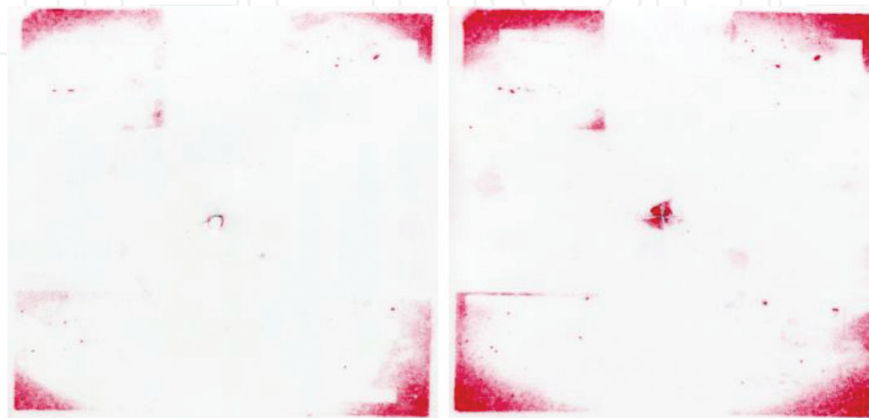
Figure 7. Pressure films for (a) four screws, 1 Nm (b) five screws, 2 Nm.
