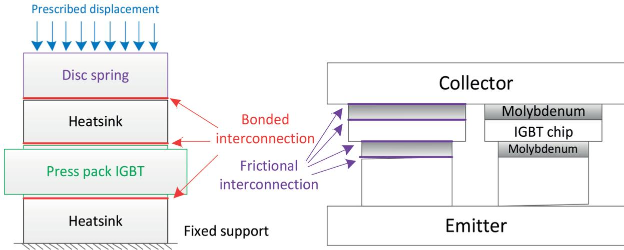
Figure 5. Boundary conditions of the mechanical model.
