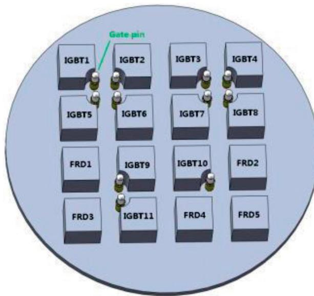
Figure 12. Finite element model and chip number.
