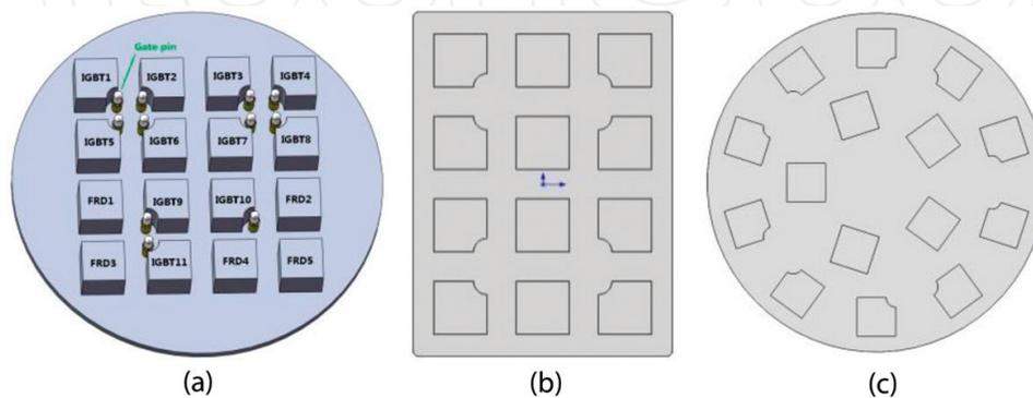
**Figure 15.** Three different layouts: (a) circular electrodes with the square internal layout, (b) square electrodes with the square internal layout, and (c) circular electrodes with the circular internal layout.
