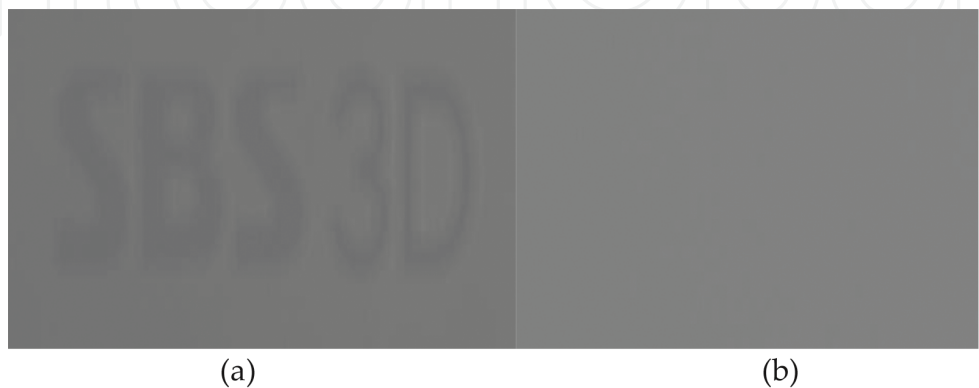
Figure 16. Image sticking test results (a) Before compensation, (b) After compensation.
