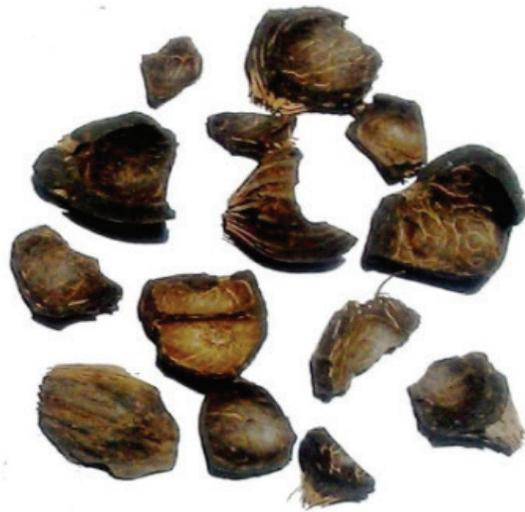
Figure 3. Different size of Oil Palm Kernel Shell for the concrete mixing.
