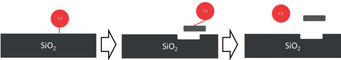
Figure 10. The schematic mechanism of oxide removal rate by ceria abrasive.
