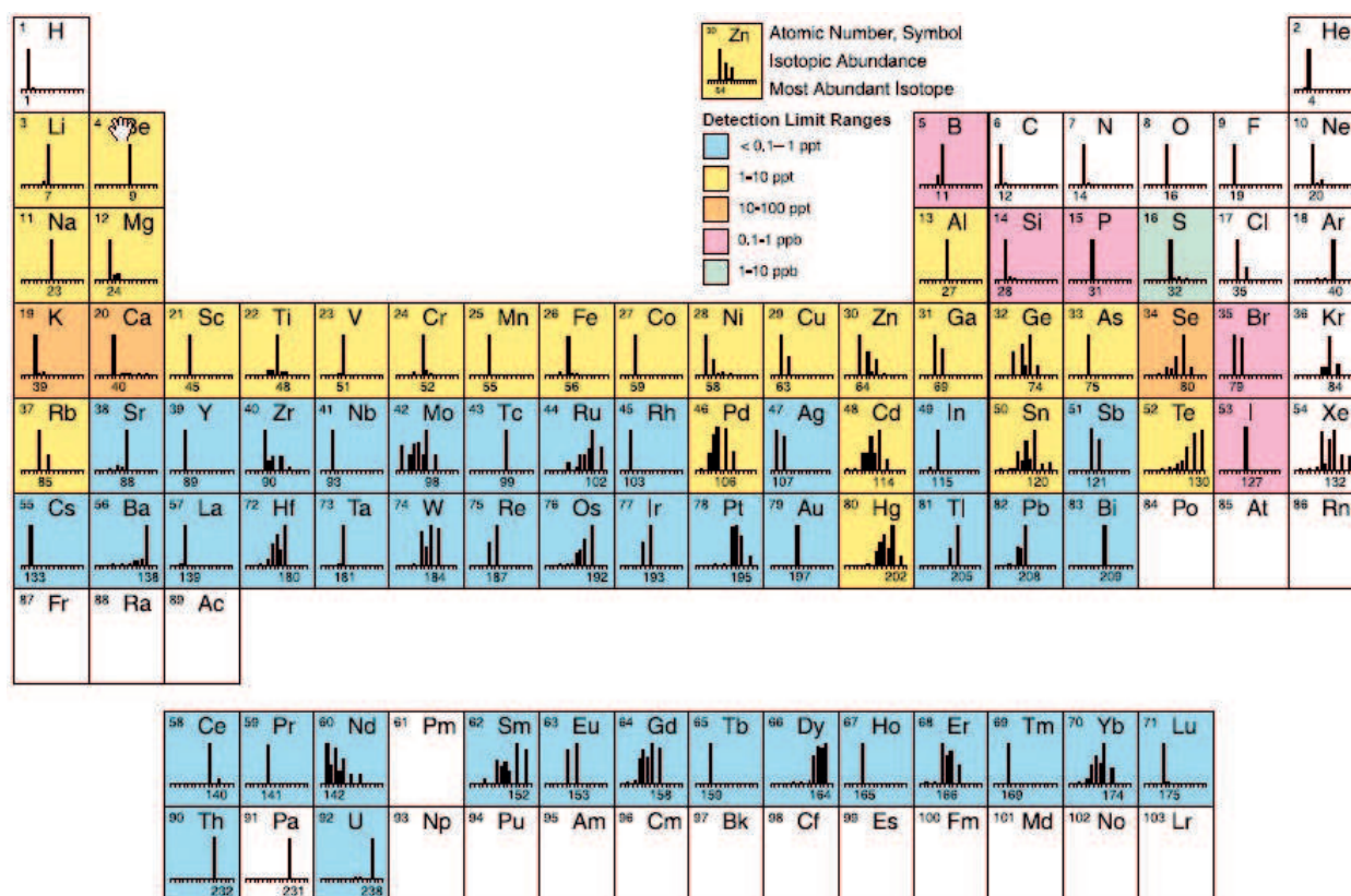
Figure 2. Elements detectable by ICP-MS analysis.
