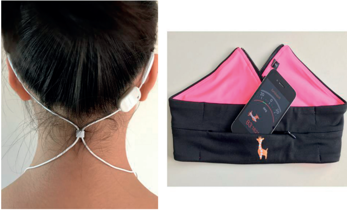
Figure 3. Posture training devices (left: head/neck training headset, right: lumbar training belt).
