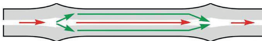
Figure 7. Configuration of a MZI constructed by two up-taper in SMFs.
