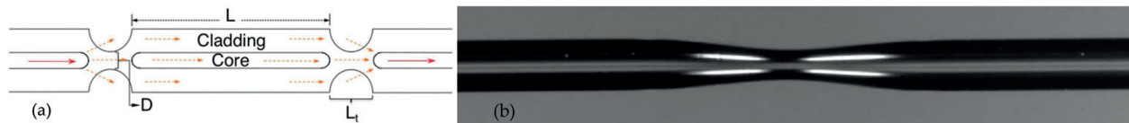
Figure 6. (a) Schematic diagram of an abrupt tapered fiber In-Line MZI; (b) microscopic image of the fabricated abrupt tapered fiber.
