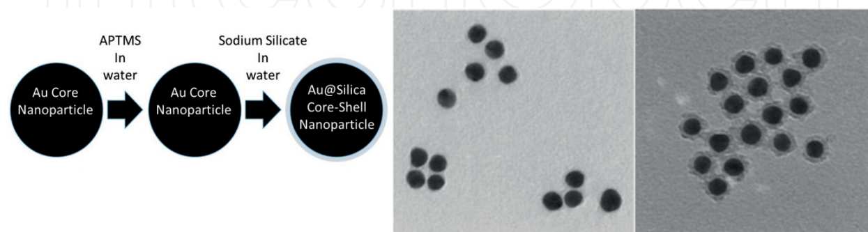
Figure 1. (Left) Schematic of aqueous synthesis procedure used by Liz-Marzán to coat thin silica shell on Au nanoparticles. (Right) TEM images of 15 nm-sized gold nanoparticles coated with 2 nm silica shells after addition of sodium silicate [6].
