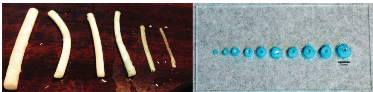
Figure 11. The models of synthetic manufactured grafts made of 10% PVA-c [17].
