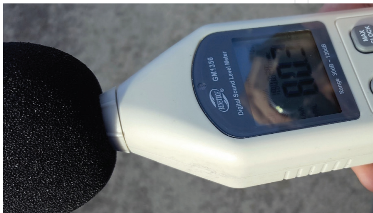
Figure 16. eKart noise intensity measurement.
