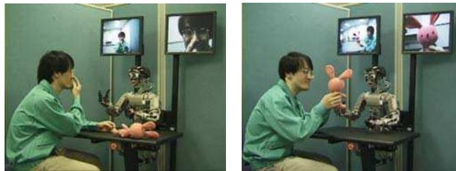
Fig. 6. Infanoid engaging in eye-contact (left) and joint attention (right).
